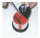
Note: If necessary, prepare the MEMOLUB® HPS with a manual grease gun (only for grease cartridges).
