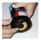
9. Simulate a function test by hand. Press the sensor pin on the bottom side of the casing for about 5 seconds.
