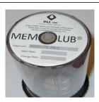
4. Remove the label from the replacement cartridge. Enter the start date and the exchange date.
