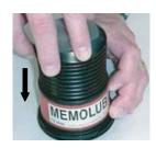
6. Turn the casing over together with the cartridge.
