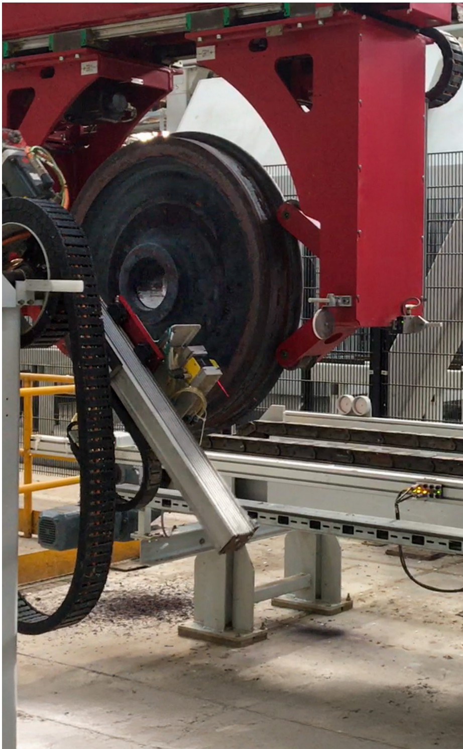
The gripper holds the wheel in front of the forged text reading station
