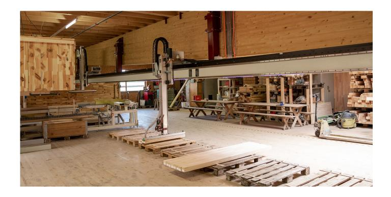
about 15 tons of material that three employees have to manually remove from the cutting machine, inspect, and then load onto the correct pallet. This is a very physical and repetitive job.
