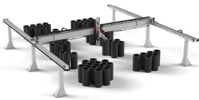
Tire and Wheel Handling: Automated solutions for handling tires and wheels from the end of curing through to shipping preparation.
